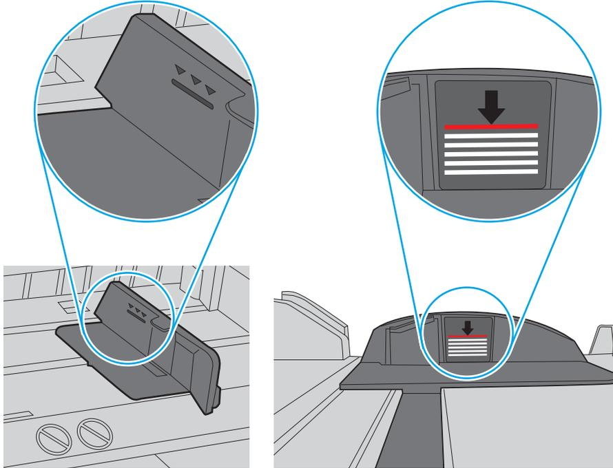
**Figure 9-7** Tab for the paper stack
