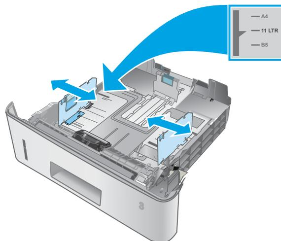
3. Adjust the paper-length guide by squeezing the adjustment latch and sliding the guides to the size of the paper being used.
