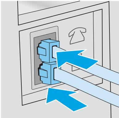
3. Remove the plug from the telephone line out port on the rear of the printer, and then connect a phone to this port.
