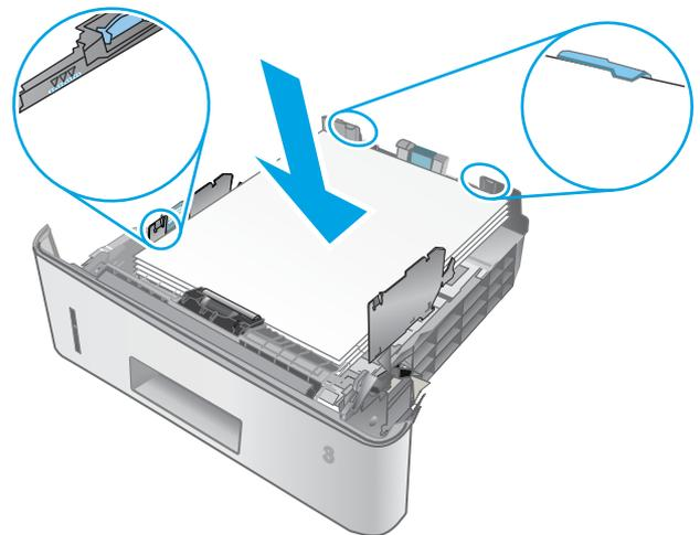
5. Slide the tray completely into the printer.
