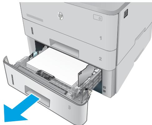
2. Remove the paper from the tray, and discard any damaged paper.
