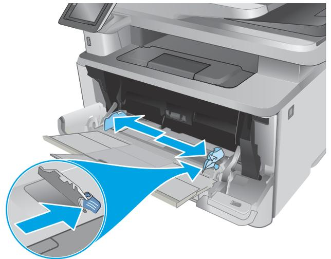
5. Load the paper into the tray. Make sure that the paper fits under the tabs and below the maximum-height indicators.
