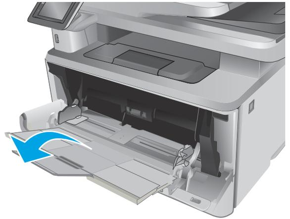
4. Press down on the tab on the right paper guide, and then spread the paper guides to the correct size.
