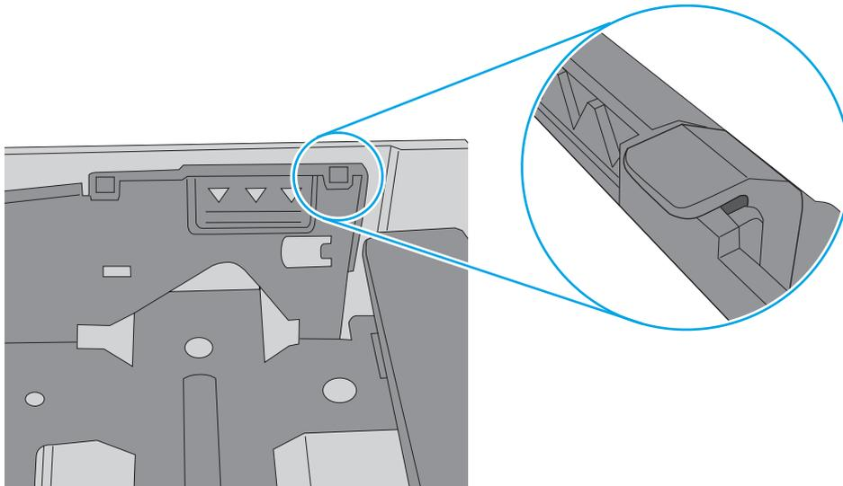
6. Make sure the paper guides in the tray are adjusted correctly for the size of paper. Adjust the guides to the appropriate indentation in the tray. The arrow on the tray guide should line up exactly with the marking on the tray.
