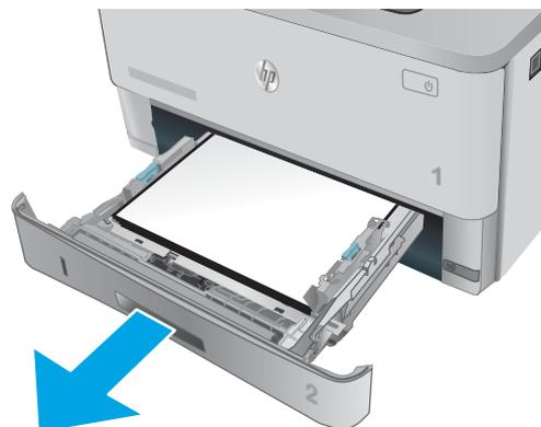
2. Remove the paper from the tray, and discard any damaged paper.
