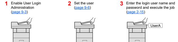
Access are in three levels - "User", "Administrator", and "Machine Administrator". The security levels can be modified only by the "Machine Administrator".
