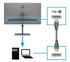
NOTE: The monitor's USB Type-C port provides network, data, video, and power delivery (up to 100 W).
