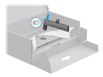
2. Attach the base to the stand (1), and tighten the screw (2).
