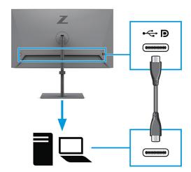
**NOTE:** Some USB Type-C ports support display output. To determine if the USB Type-C port on your monitor is capable of supporting DisplayPort output, see <a href="Rear components on page 4">Rear components on page 4</a>.
