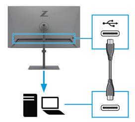
NOTE: The monitor delivers up to 100 W of power over a USB Type-C connection. When connecting the host computer via USB Type-C, DC power out does not need to be connected. Do not connect two power sources (DC power in and USB Type-C) to the host computer.
