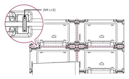
2 Complete the 2 x 2 tiling. You can use various options of tiling including 3 x 3 by using the same method.
