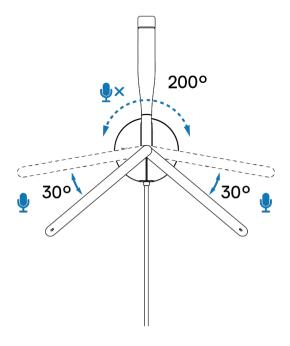
CAUTION: To avoid breaking the boom microphone, do not rotate over ±130°.
