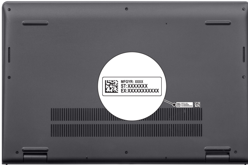
Figure 7. Service Tag/Express Service Code location
