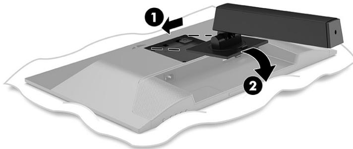
The latch on the bottom of the mounting plate pops up when the stand is locked in place.
