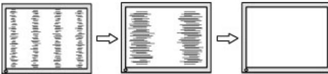
3. After adjusting the Clock, if flickering, blurring, or bars appear on the screen, proceed to adjust the Phase.
